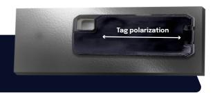
clean and dry the surface for obtaining the maximum bond strength. Ideal application temperature is from +21°C to +38°C (+70°F to +100°F), bond strength can be improved with firm application pressure and moderate heating from +38°C to +54°C (+100°F to +130°F). Installation at temperatures below 10°C (50°F) is not recommended.
